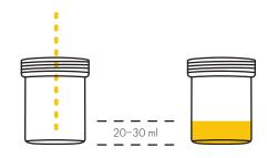
Perform a first catch (sample collected from initial urine stream). Collect between 20-30 ml. Check to see the urine volume. IMPORTANT: Only fill the urine cup up 25% of the way, between the 20-30 ml mark only. Collections larger than 30 ml may result in specimen dilution which may reduce test sensitivity or result in sample rejection. The 30mL mark is at the bottom of the frosted label.
