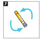
Invert the tube 8-10 times to mix the specimen.
